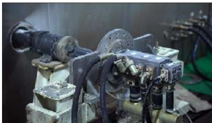
Hydraulic oil pump Low-temperature performance test under -40
